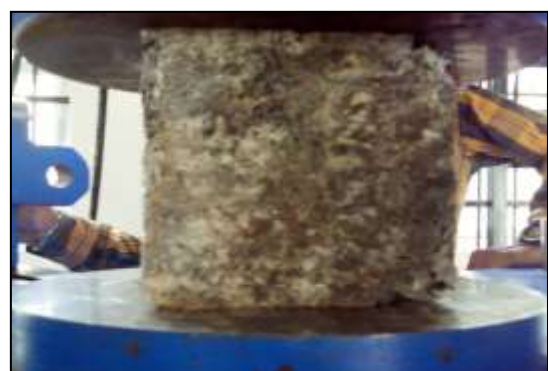
FIG. 3 COMPRESSIVE STRENGTH TESTING OF GFRHSC CUBE
